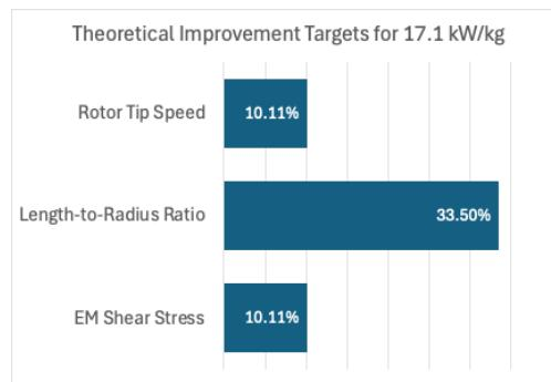
The major trade space in the design of an electrical machine is between power and specific power. The idealized specific power formula asserts that  $SP \sim P^{-\frac{1}{2}}$ . However, this neglects the fact that the optimal or achievable EM shear stress, length-to-radius ratio, and tip speed change with the power of the machine. In a sequence of optimizations performed by Dowdle, it was
