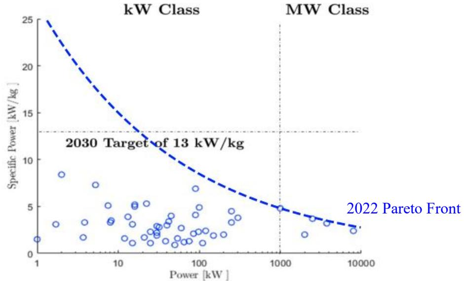
The achievement of a 1 MW machine with a specific power of 17.1 kW/kg by the MIT GTL in 2025 can be seen as a shift in this pareto front:
