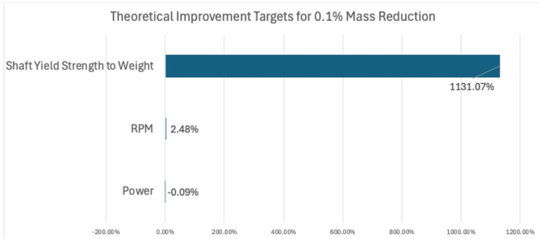
This tornado chart is dominated by the lack of sensitivity of mass to shaft structural efficiency. The mass of the system is by far the most sensitive to the power.
